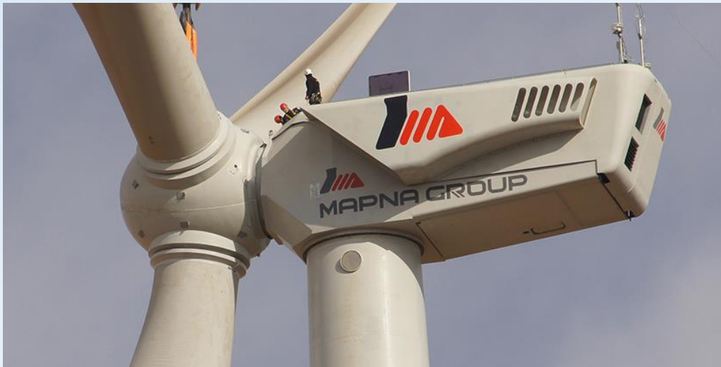
Wind Turbine 2.5 MW
